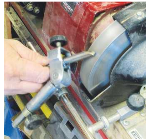
▲ Pic.18 Always use a freshly sharpened tool at this stage. Les finds the Tormek bench grinding jig is really precise and easy to use
